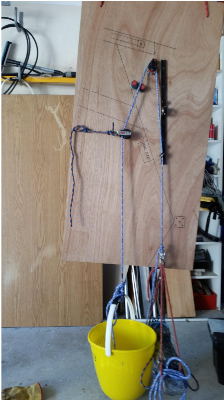
The test harness for determining the holding power of the ratchet block.
