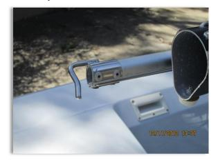
The ideal pole set up is a parrot beak at one end and "Douglass Pin" at the other. This makes gybing much simpler. Ideally ensure that the pin that attaches to the mast is not too deep as this makes getting it place, especially after gybing the jib, much harder.
