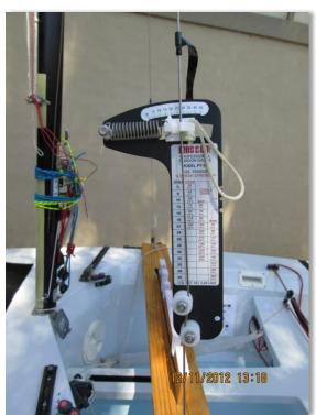
the newer Ronstan RCB system (the new tracks have slightly more range). If the wind increases a slight stay adjustment will give you 22 (24 on RCB system) on your Loos gauge. More than enough for the upper limits of the class.
