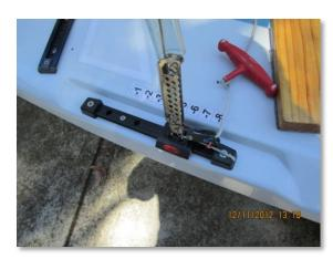
The standard setting, which gives you range from 0-18/20 knots (exact range depending on crew weight) is measured with the rig pulled fully back.
