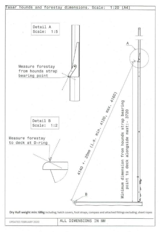
Mast and Rigging Measurement Diagram
