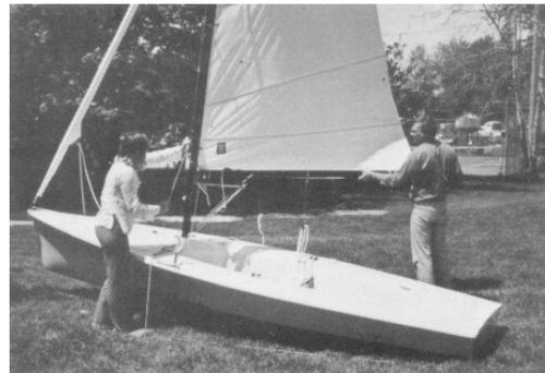
**40.** When the sail is nearly at the top, lift the boom off the gooseneck pin; it helps if one person holds the boom up to take its weight off the sail. Loosen the vang, because if it is tight, it will hold down the end of the boom and raising the sail to the top will be impossible.
