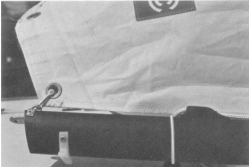
**37.** Attach the tack of the sail to the boom at the forward end with a shackle.
