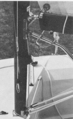
**42.** When the halyard is locked at the top of the mast, pass the loop of the shockcord under the small black hook and remove the rope tail completely.
