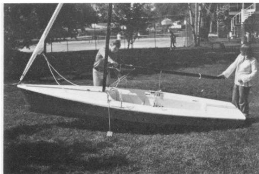
**32.** The first time you rig your boat, have your crew hold the end of the boom level to the ground and make sure the boom vang and mainsheet ropes are correctly reeved before hoisting the sail.
