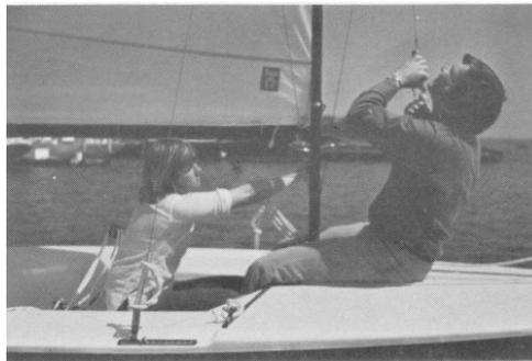
**57.** In order to put the ball into the halyard lock, use the rotation lever to turn the mast at right angles to the person on deck. At this point the halyard lock will be directly overhead. (Remember this also for lowering the sail — use the lever to make the halyard lock accessible and then re-align the mast with the sail so that it will come down smoothly.)
