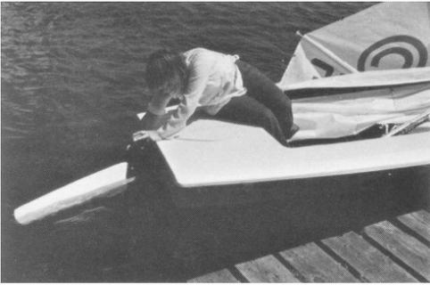
**53.** Make sure you push the rudder all the way down until the spring clip locks under the top gudgeon. Note that the blade is in the up position requiring no depth of water. Do not install the tiller yet as it will only tend to catch the sail while hoisting.
