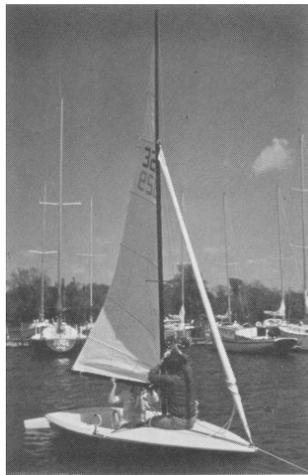
**56.** When the sail is almost all the way hoisted, the person in the cockpit should assist by raising the entire boom to take its weight off the sail.
