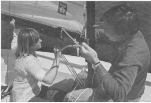
**58.** A hint for windy days. Pull the outhaul very tight to make sure the sail is completely flat. This greatly reduces the tendency of the boom to flog from side to side.
