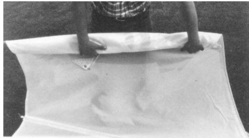
Fold the sail at the second or third batten and roll down to the boom. Never roll the sail around the boom, (boom fittings mark or damage the sail).
